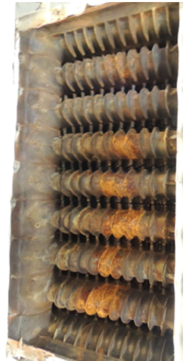
Multiple sections fractured
