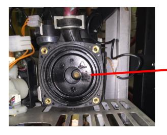
Pump motor removed from housing. Be sure gasket comes out with bad motor or remove from housing. Make sure new motor has new gasket in place before installing.
