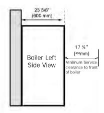
FIGURE 4-2c Combustible Clearances - Closet Installation
