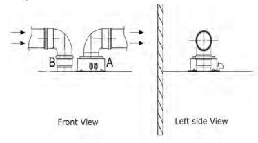
FIGURE 6-6 - Separated Horizontal Flue Termination
