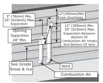
FIGURE 6-9 Two Pipe Side Wall Vent (Multiple Appliances).
