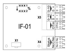
4. Analog Temperature-Based Control - 0 - 10 V signal controls boiler supply temperature between 32°F (0°C )and 176°F (80°C). Control modulates on basis of supply temperature, heat output varies between minimum and maximum values based on supply temperature set point calculated by the controller. Jumper 2 on the interface is used to select either temperature control ( ) or heat output control (%).
