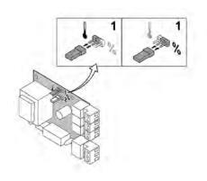
**6.** Analog Output - 0-10V - Temperature or heat output can be chosen for this feedback message. The two controls are described briefly below. Jumper 1 on the interface is used to select either
