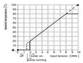
5. Analog Heat Output - Based Control - 0-10V signal controls boiler output between 0% and 100%. Minimum and maximum values are limited. Minimum output is linked to boiler's modulation depth. Output varies between minimum and maximum value on basis of value determined by controller.
