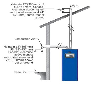
Fig. 6-12 Flue on Sidewall, Combustion Air on Roof
