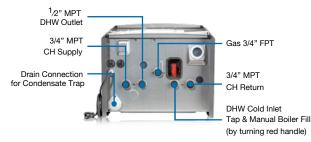
The piping connections on the boiler are all straight thread and not tapered. The required adapters are supplied with the boiler for field installation.
