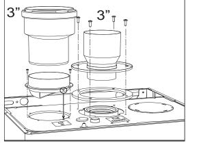
Horizontal Venting requires field supplied appliance adapter for the boiler flue outlet. Boiler is provided with a 3" vent connection, 3"
