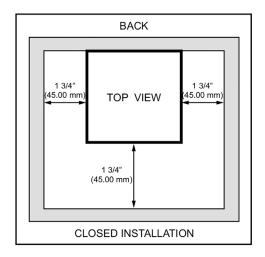
**0 in /0 mm** between the Back of the Unit and the wall CLOSET INSTALLATION
