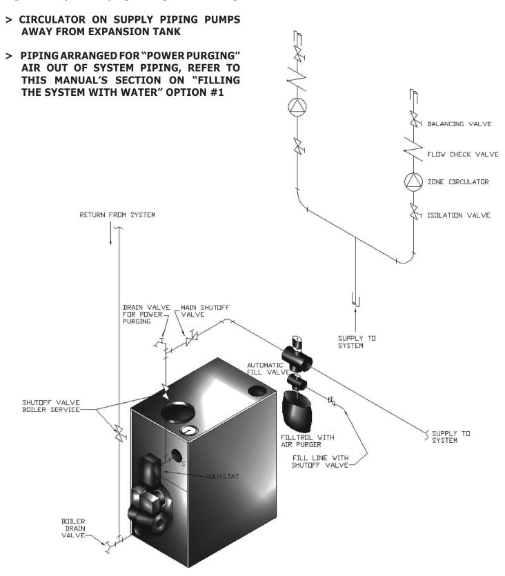
Figure 10 - System Piping Arrangement Alternate Near Boiler Piping
