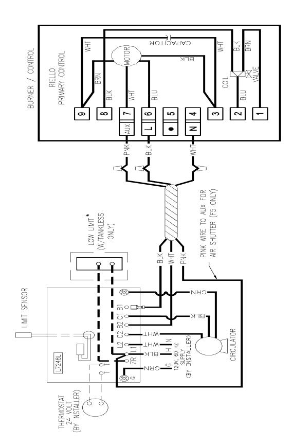
\* When Low Limit Is Used, Set ELL Parameter On L7248 Honeywell Control To On. Boilers Factory Equipped With Tankless Coil Are Factory Set To On.
