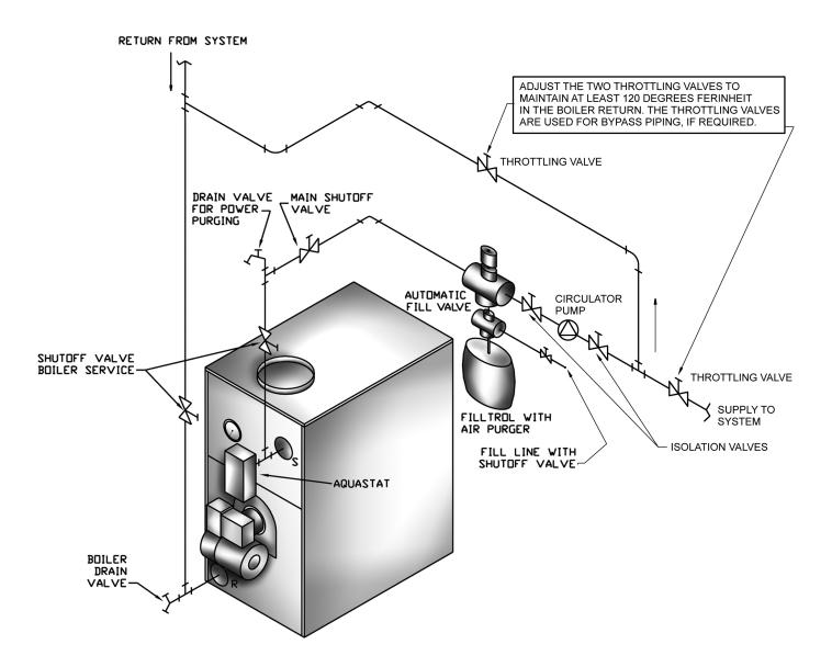
Figure 8 - System Piping Arrangement Zoning With Zone Valves
