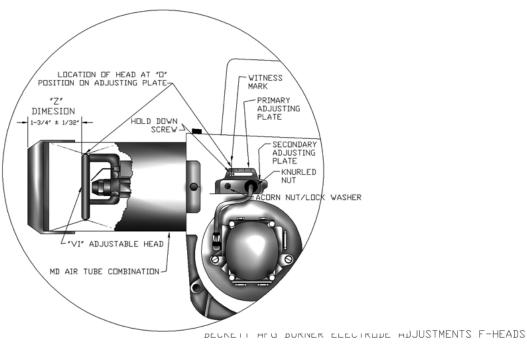
BURNER F-HEAD MODEL DIMENSION 'N' (HEAD TO NOZZLE)
