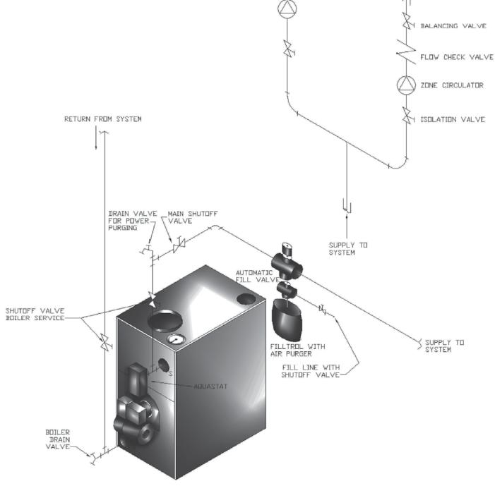
Figure 10 - System Piping Arrangement Alternate Near Boiler Piping
