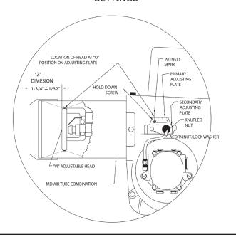
Figure 17 - Riello Turbulator Setting
