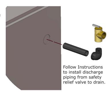
Figure 6b - Discharge Piping From Safety Relief Valve
