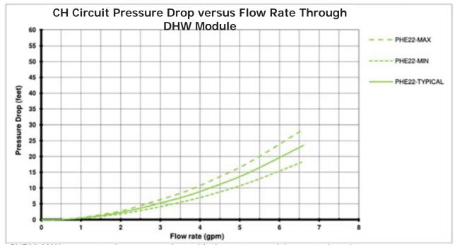
PHE22-MAX represents the pressure drop with the motor at minimum stroke tolerance.
