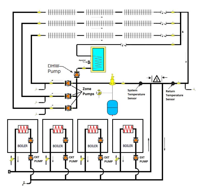
**NOTE:** Manufacturer requires all domestic hot water (DHW) installations use an anti-scald valve. Local codes may require additional equipment (expansion tank, relief valves, etc.) Select and size equipment to suit installation and meet code requirements.
