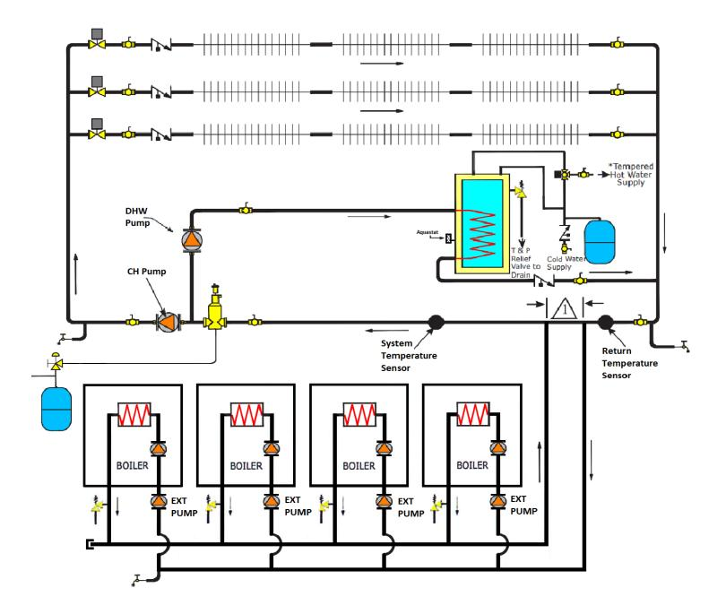
**NOTE:** Manufacturer requires all domestic hot water (DHW) installations use an anti-scald valve. Local codes may require additional equipment (expansion tank, relief valves, etc.) Select and size equipment to suit installation and meet code requirements.
