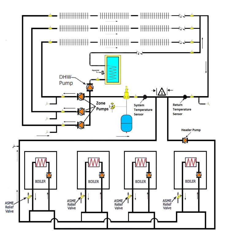
**NOTE:** Manufacturer requires all domestic hot water (DHW) installations use an anti-scald valve. Local codes may require additional equipment (expansion tank, relief valves, etc.) Select and size equipment to suit installation and meet code requirements.
