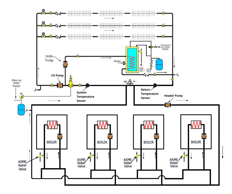
**NOTE:** Manufacturer requires all domestic hot water (DHW) installations use an anti-scald valve. Local codes may require additional equipment (expansion tank, relief valves, etc.) Select and size equipment to suit installation and meet code requirements.
