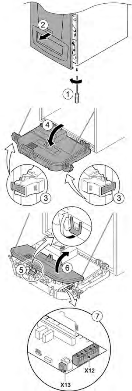
FIGURE 8-2 Remove Front Panel
