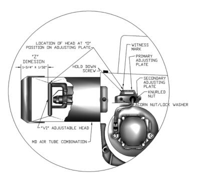
BECKETT AFG BURNER ELECTRODE ADJUSTMENTS F-HEADS
