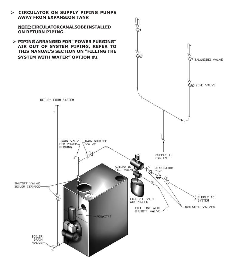
Figure 9 - System Piping Arrangement Zoning With Circulators
