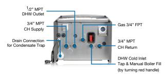
The piping connections on the boiler are all straight thread and not tapered. The required adapters are supplied with the boiler for field installation.
